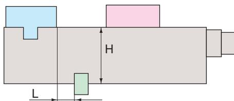
H寸法公差 **0.01**mm 以内 H-dimension tolerance **0.01**mm or less
