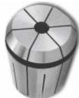
Premium / HP - High Precision Collet (.0002"/5 micron TIR) (.020/.5mm collapse range)
