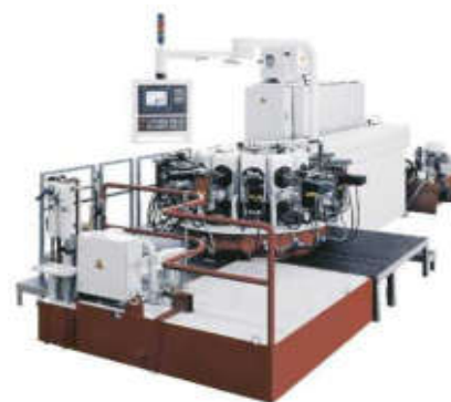
Machines Transfert - Transfert Maschinen Transfer Machines
