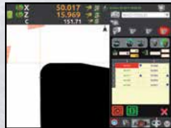
Automatic measurement detects the highest values in X and Z to ensure the most accurate representation of the cutting tool.
