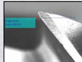
Cylindrical cutter with 4 cutting edges, diameter 6mm. Side view (chest): measure the propeller screw angle and rake angle, important to determinate to suit the type of application and the type of material being processed.
