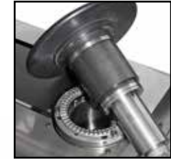
Mechanical Draw Bar clamping with any retention knob.
