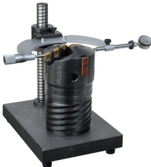
botek setting gauge, measurement range 100 - 600 mm
